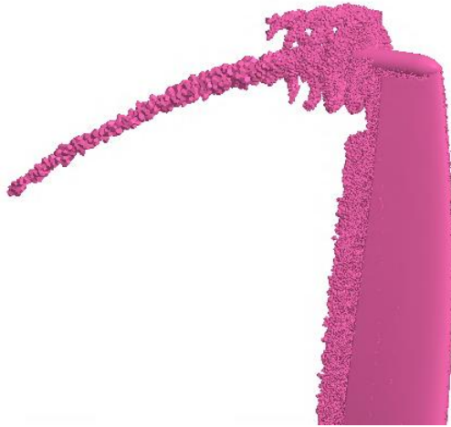
Figure 16. Vorticity threshold visualization from combined-stage CFD highlighting tip vortices shed from both the main rotor and secondary rotor
